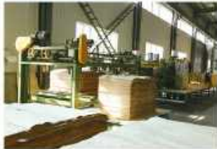
Veneer jointing machine
